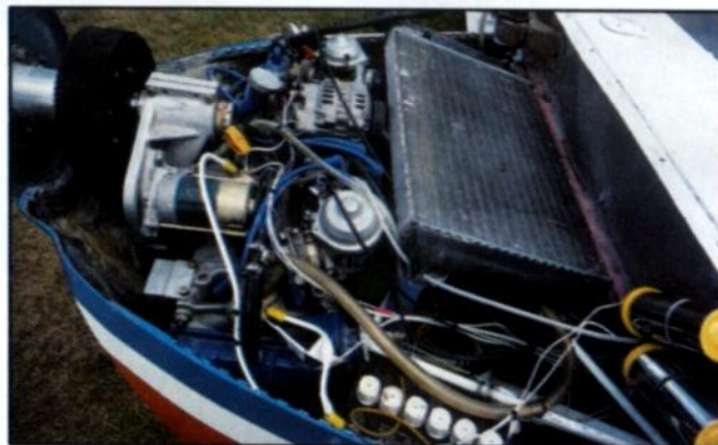
The Vision prototype is powered by a 100-hp Subaru EA-81.
